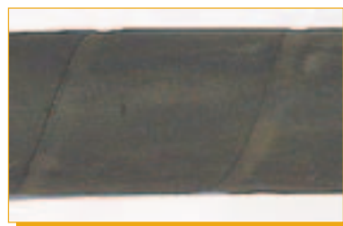
Figure 9. The print left by the bandaging is clearly visible on this finished non-Watson-Marlow Bredel hose.
