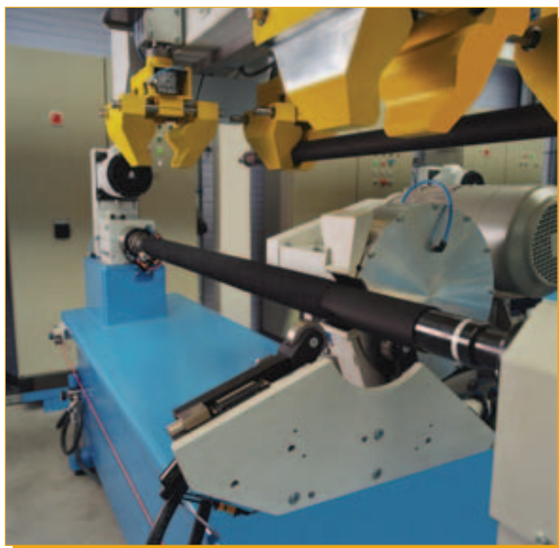
Figure 8. The outer surface of Watson-Marlow Bredel’s hoses are ground to a uniform wall thickness.
